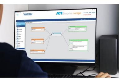
One of the key features of the latest version of ACT is the use of **rules mapping** to enable advanced configurations of triggers. These can be actioned on events such as system input and output change, and card swipe outcomes across the access control system as well as other elements of an integrated system such as intrusion system events.
