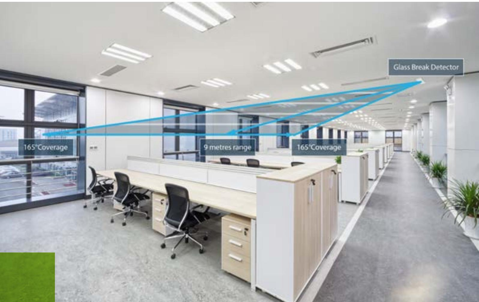
The AGB800-AM, has the same solid foundation of the AGB800, with the added functionality of anti-mask. At the time of writing the AGB800-AM is the only acoustic glass break detector to pass the rigorous requirements of EN50131-2-7-1:2013, Grade 3 for high security installations. The AGB800-AM anti-mask functions provides unique tamper protection, which is signaled via a separate relay.
