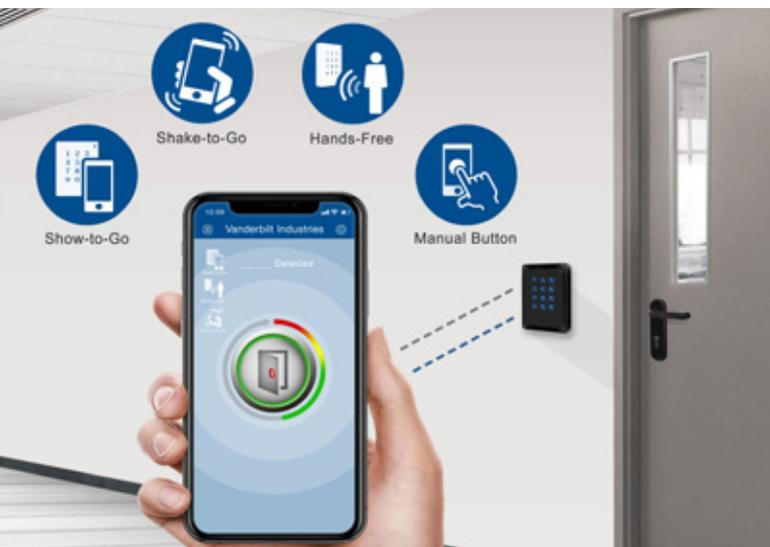
Reading distances are a key factor for Bluetooth access control. Our user-friendly Mobile APP offers a unique four identification option: "Shake to Go," "Show to Go," "Manual Button Mode," and "Hands-Free Mode," which allows users to select a mode best suited to their needs. Bluetooth readers also allow the use of conventional access cards and support 13.56MHz standards.
