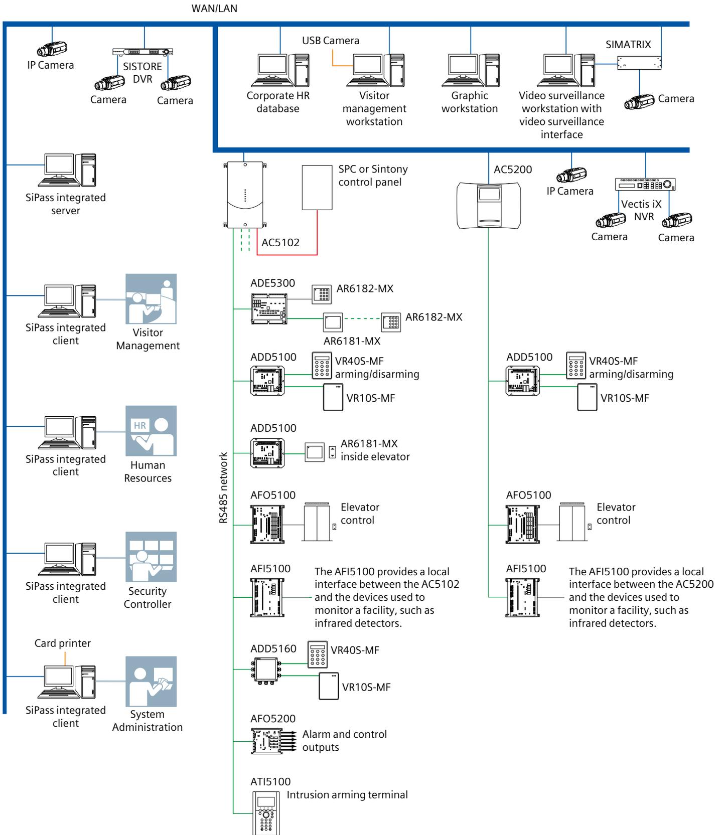
SiPass integrated is fully customized to meet the needs of the organization at which it is installed. It can be set up to monitor entries only, or both entries and exits (anti-passback), and/or it can be used to control the operation of elevators. Areas of a building that have a higher security requirement than others can be secured with video surveillance technology.
